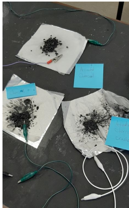
Three different batteries; one with granular activated charcoal, crushed activated charcoal, and non-activated charcoal (a crushed charcoal briquette).
